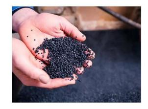
This sustainable plastic granulate is EUCert-Plast certified because 80% or more of the granulate consists of recycled raw materials.
